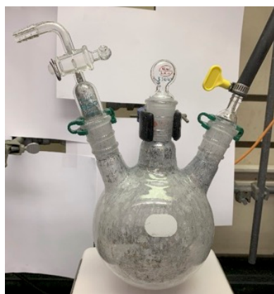
Figure 11. Li-dendrites scraped down. (photo provided by the checkers)
