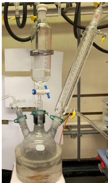
Figure 12. Addition funnel and reflux condenser (photo provided by checkers)
