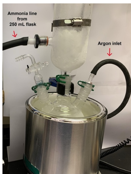
Figure 5. Reaction flask submerged in dry ice-acetone bath prior to ammonia transfer.
