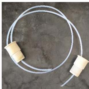
Figure 14. PTFE tubing fitted to rubber septa (photo provided by the submitters)
