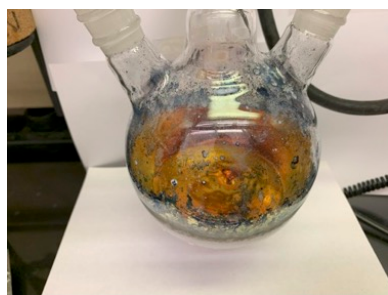
Figure 7. Bronze-colored solution of lithium in ammonia. (photo provided by the checkers)
