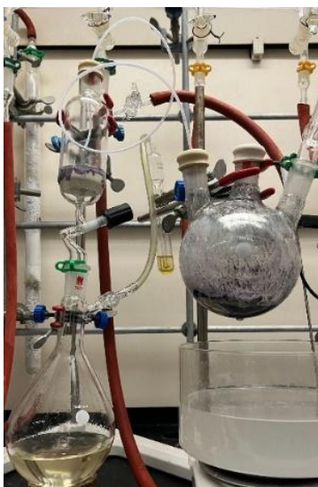
Figure 17. Filtration setup (photo provided by submitters)
