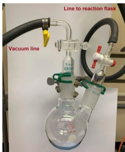
Figure 8. Secondary liquid N 2 trap (photo provided by the checkers)
