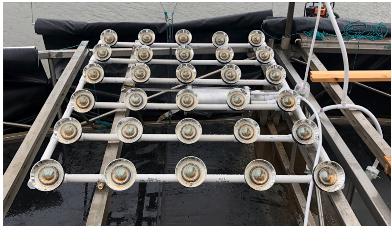
Fig. 12. Completed Nikhef plane installed in the detector. Each PMT has an acrylic cover and reflector attached. The PMTs are sealed inside their inserts and installed into the PVC plane frame. The electronics container located in the centre of the plane. A flexible PVC hose (incomplete) exits the electronics container, which would connect the plane to upstream power supplies and DAQ electronics.
