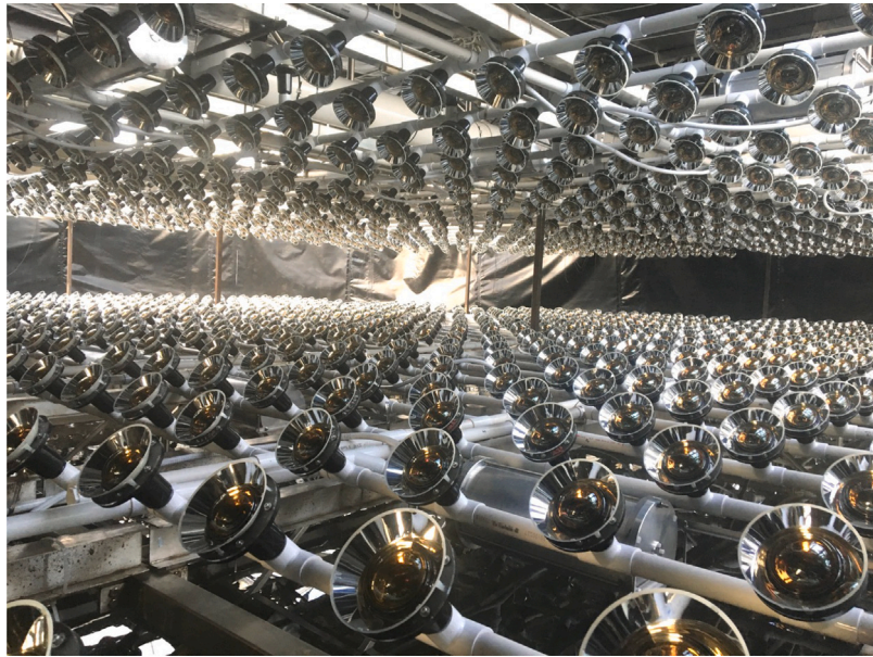
Fig. 16. The interior of the detector: the rows of Nikhef PMTs angled to point into the neutrino beam can be seen. The narrow height between the bottom and top caps before the expansion during deployment is visible. Image courtesy of Albrecht Karle.
