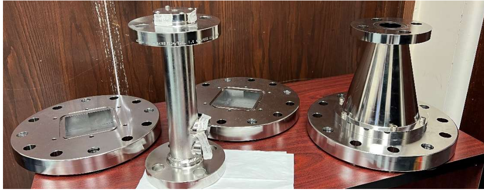
Figure 99: Detonation Tube II Turbulator Section, Expansion Section and Flanges
