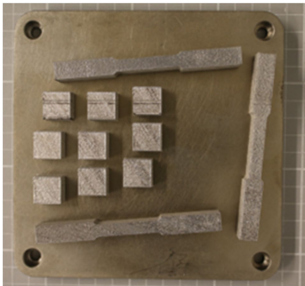
Fig. 4 Gaussian distribution build: nine cubic and three tensile specimens manufactured by LPBF
