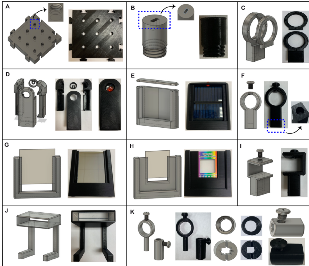
Figure 1. 3D design and printed components: (a) modular optical breadboard featuring screw-in holes compatible with \frac{1}{4} inch screws. The insert highlights the arrangement of screw holes. (b) Breadboard pegs. (c) Optical mounts. (d) Mounts specifically designed to accommodate LED circuitry and an 9 V battery. (e) Mount crafted to encase the solar cell circuitry along with an LED indicator. (f) Mount tailored to accommodate a flashlight or laser source of 38 mm diameter. (g) Mount engineered to hold a 75 mm \times 75 mm reflective mirror. (h) Mount designed to house a 51.50 mm \times 51.25 mm diffraction grating. (i) Rectangular prism mount with a cross-sectional width of 26.15 mm. (j) Mount crafted to encase the rectangular prism (k) components include a height-adjustable laser mount, circular and rectangular PCB holders, and a laser holder with adjustable diameter for precise laser source positioning and PCB handling.
