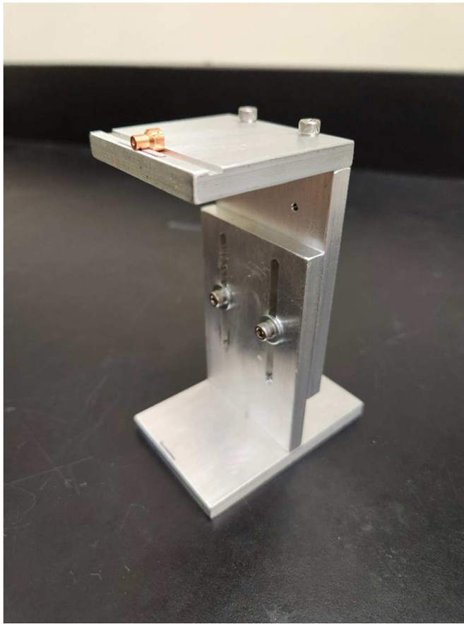
Fig. 1. Cathode holder designed for use in the gamma counting station. The cathode sits in the groove, facing outward and the stand can be adjusted by loosening the two set screws and moving the top piece up or down.
