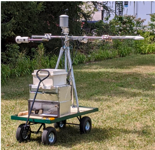
Fig. 1. The mobile human-biometeorological platform ( MaRTy cart) designed to gather pedestrian thermal exposure data in Guelph, Canada during summer and winter (left). Sensors used on MaRTy for each variable, associated specifications, and the height each sensor is mounted (right).
