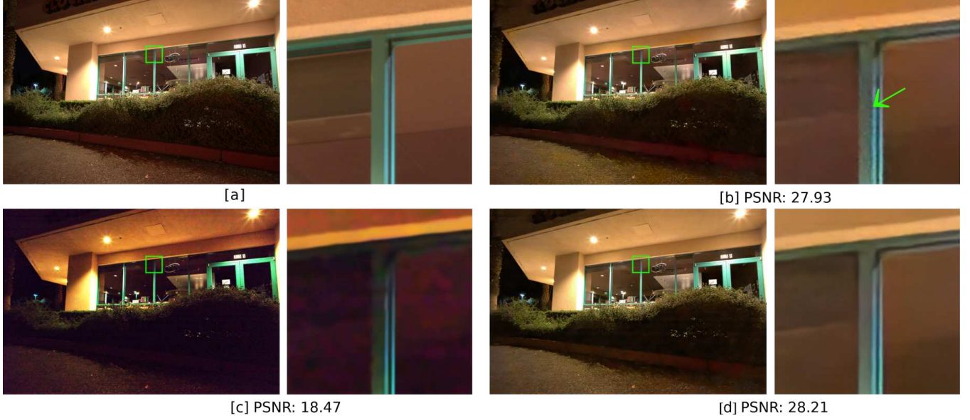
Fig. 3: Image denoising results. [a] Ground truth image. [b] Output from SID. Noise is still present in few parts of the image. [c] Output from BM3D. Denoised image is darker than the ground truth. [d] Denoised output from our network.
