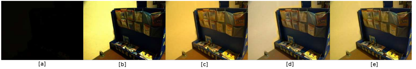
Fig. 4: Comparison of color Accuracy. [a] Input dark image. [b] 100x scaled version of dark images. [c] Ground truth with exposure time of 10 seconds. [d] SID output with missing color information, PSNR: 20.48dB. [e] Output from our network with close approximation to ground truth image, PSNR: 27.17dB.
