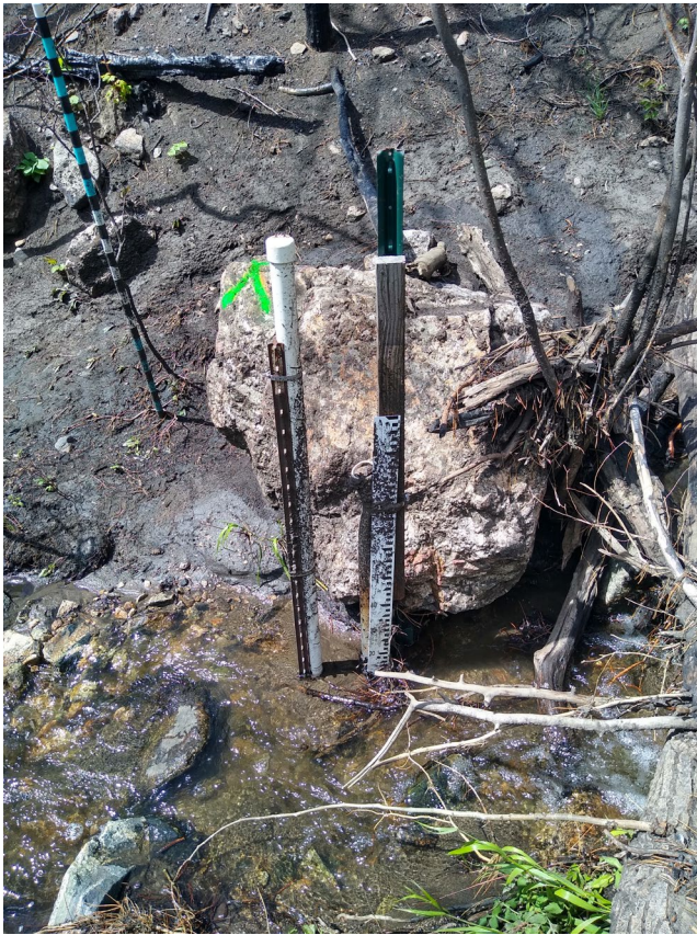
FIGURE 9 | Geomorphic change observed at severely burned, low snow zone. After a large rainstorm on June 25, 2021, the stream sensor was covered with ~10 cm of fine sediment. The debris marking the upper levels of the staff plate implies that a large amount of sediment was moved downstream. Photograph courtesy of Stephanie Kampf.
