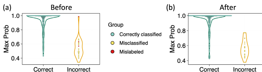
FIGURE 5 | Maximum predicted probability for correctly and incorrectly predicted samples of all diblock copolymers using the physics-informed features for (a) the original samples; (b) revised samples after correcting three mislabeled detected by our method.
