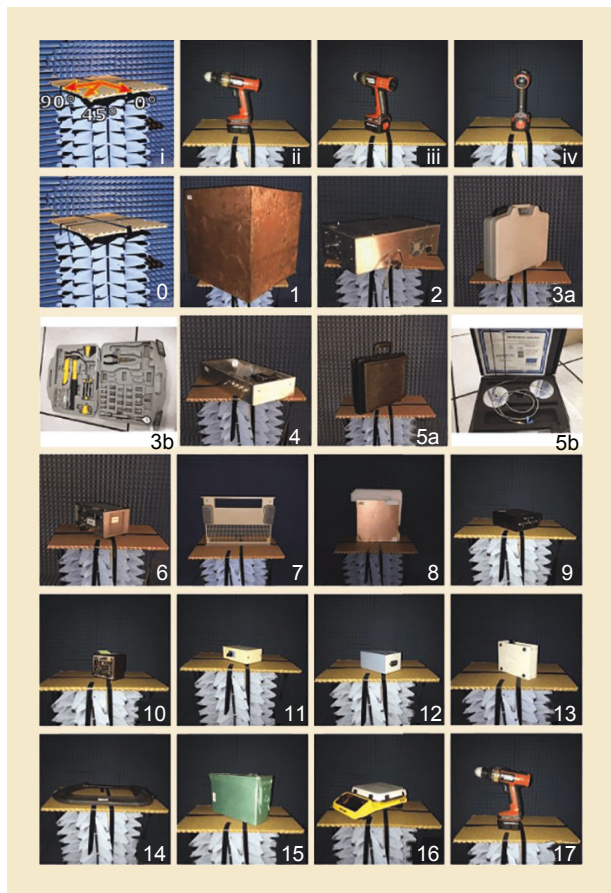
FIGURE 5. The 17 targets are shown on the platform. Object size can be gauged by the 47-cm-wide and 30.5-cm-deep cardboard platform. The 0°, 45°, and 90° orientations are shown in (ii), (iii), and (iv), respectively. The red arrows depict the orientations on the cardboard. Unless otherwise noted, the photos are taken from the radar's perspective at a 45° orientation. The objects vary in size and composition, affecting the rRCS. (0) Platform: Roughly 60° from the radar's perspective. (1) Object 1: An empty metal (copper) box with a hole on the top face. (2) Object 2: A metal box (closed cover) with a home-built circuit. (3a) Object 3: A plastic toolbox (closed). (3b) Object 3: Open. Data were collected with the toolbox closed. (4) Object 4: A metal box (open cover) with a custom circuit. (5a) Object 5: A plastic box (closed). (5b) Object 5: Open. Data were collected with the box closed. (6) Object 6: A dc power supply (metal cover). (7) Object 7: The front cover of a power amplifier (metal) at 90° orientation. (8) Object 8: Rogers duroid laminate (copper) at 90° orientation. (9) Object 9: A data transfer switch box (with a plastic cover). (10) Object 10: A variable capacitor box (with a metal cover). (11) Object 11: A data transfer switch box (with a metal cover). (12) Object 12: A port converter (metallic). (13) Object 13: A data transfer switch box (with a plastic and metal cover). (14) Object 14: A vise (metal) at 0° orientation. (15) Object 15: A metal box. (16) Object 16: A chemistry hotplate stirrer. (17) Object 17: A Black & Decker drill at 0° orientation.
