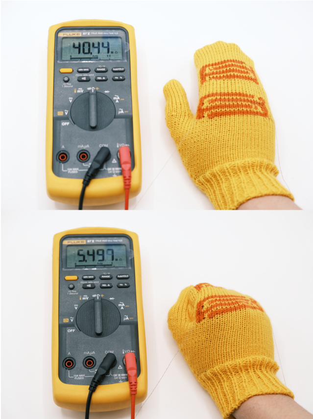
Figure 19: Knit bend sensors: The interdigital electrode structure used for the sock shown in Figure 16 can also be used to sense stretch, used here as part of a bend-sensing mitten.
