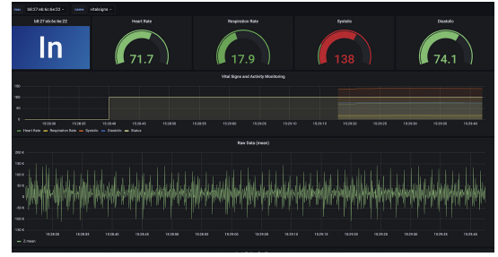
Fig. 12. Sleep monitoring GUI, that is able to visualize vital signs, such as HR and RR.
