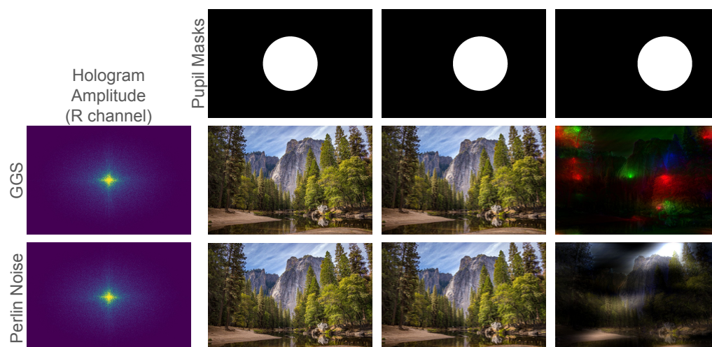
Figure 15. Eyebox comparison between GGS and Instant-SFH with Perlin-noise-based phase at 80% sparsity. The pupil mask (top row) shows the pupil moving progressively to the right. The center row shows images reconstructed from GGS. The bottom row shows images reconstructed from Instant-SFH using Perlin noise.
