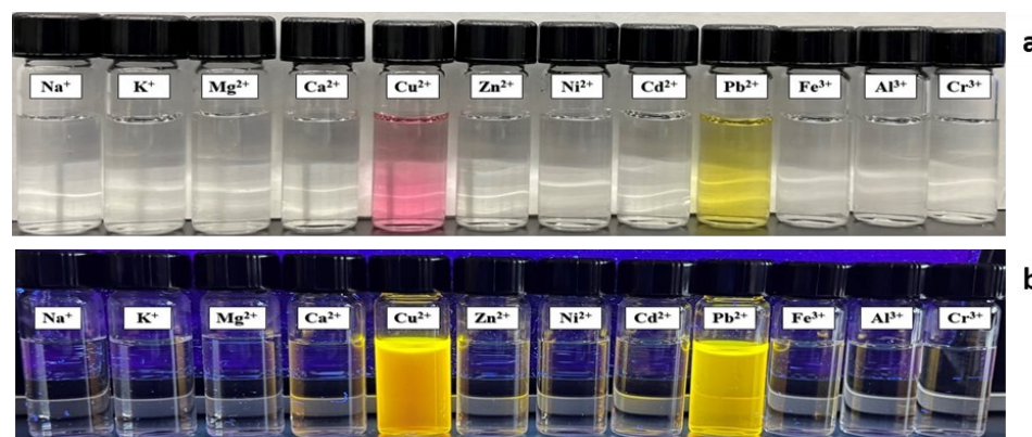
Figure 2. The visual color of sensor RdN (a) and the fluorescence under UV illumination after adding various metal ions (b).
