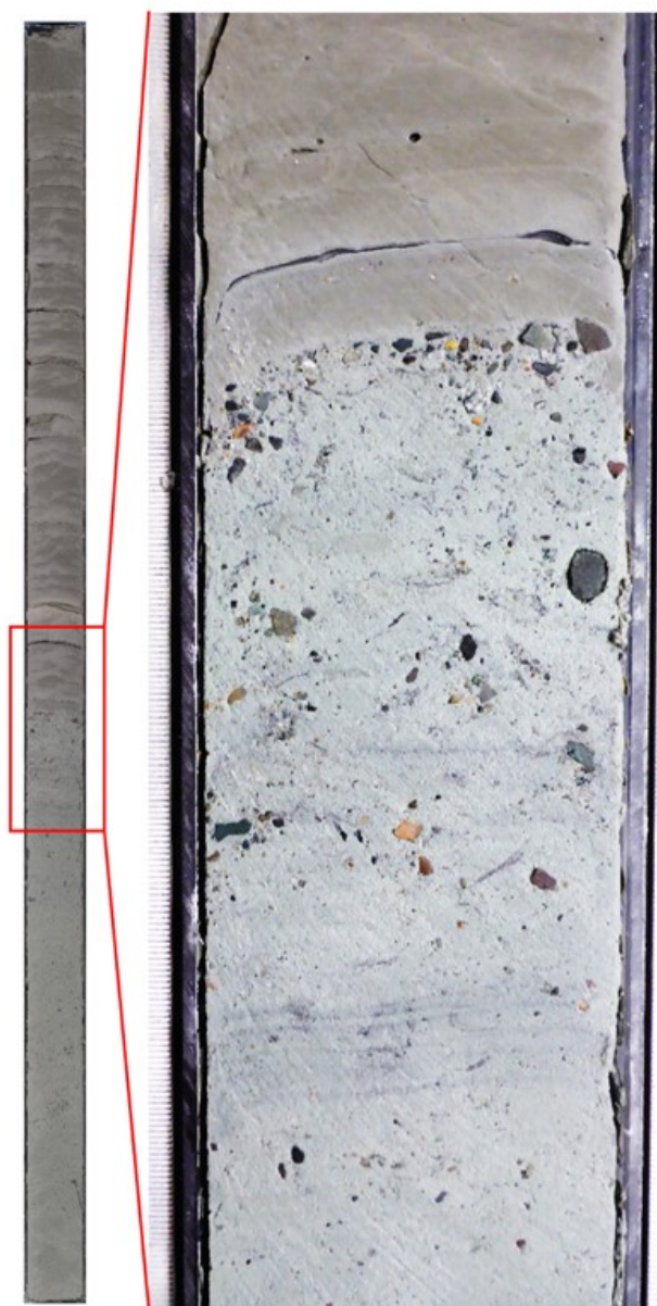
Figure 11. Core photo of a section of U1533B-14H-1 (140.24–140.44 m b.s.f.) showing correspondence of IRD and diatomite late in a Pliocene interglacial, with a sharp rapid transition, likely erosional, to overlying laminated silts. The light-colored sediments are altered diatomite. Diagenetic alteration of the diatoms precluded the detailed examination that was performed on U1532C-6F.
