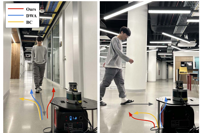
Fig. 1. The trajectories of VLM-Social-Nav (red), DWA (blue), and BC (yellow) approaches in the frontal encountering scenario (left) and the intersection scenario (right). The resulting trajectories show that VLM-Social-Nav demonstrates more socially compliant behavior because it is instructed by a prompt.
