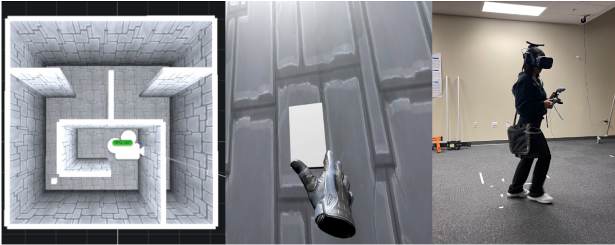
Figure 1: a) Top-down view of a randomly generated virtual maze environment b) First-person point of view - a participant grabs the trophy to start another random maze task c) Participants physically walked in the real environment to enable virtual environment navigation
