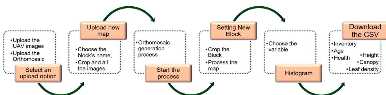
Fig. 2. Workflow from uploading UAV images to generating the final results on Agroview.
