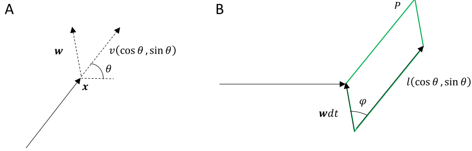
Fig. 7. Vector geometry used in the estimation of the MFP. (A) Rod at \mathbf{x} where \mathbf{e}(\theta) = (\cos \theta, \sin \theta) moves with velocity v\mathbf{e}(\theta) . In the reference coordinates of a horizontally moving rod with velocity (v, 0) , the rod velocity is \mathbf{w} . (B) A rod moving horizontally to the right, during time interval [t^*, t^* + \Delta t] can collide with a rod which has orientation \mathbf{e}(\theta) whose center is located in the parallelogram P , formed by vectors \mathbf{w} \Delta t and l\mathbf{e}(\theta) . The area of the parallelogram equals |\sin \phi| v l \Delta t .
