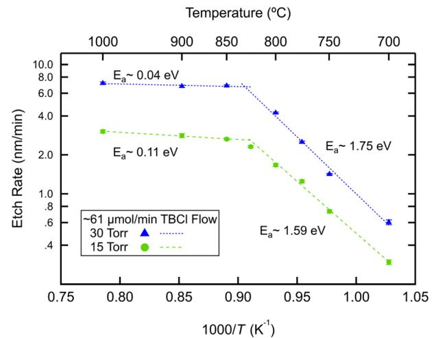
**FIG. 2.** Arrhenius plot of *in situ* etch rate of heteroepitaxial  $\beta\text{-Ga}_2\text{O}_3$  for a TBCl molar flow of  $\sim$ 61  $\mu\text{mol}/\text{min}$  at reactor pressures of 15 and 30 Torr. The HT and LT etch regimes are delineated by distinct apparent activation energies.
