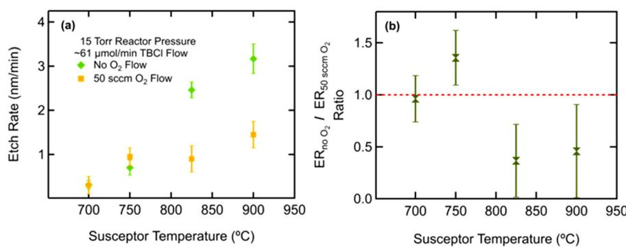
**FIG. 4.** Effect of additional  $\text{O}_2$  flow on the etch rate. (a) Etch rate as a function of susceptor temperature with no  $\text{O}_2$  (green) and with 50 sccm  $\text{O}_2$  flow (yellow). (b) Ratio of the etch rate without oxygen divided by the etch rate with oxygen vs susceptor temperature. Below 800 °C, the etch rate is relatively unchanged, but it is suppressed at higher temperatures.
