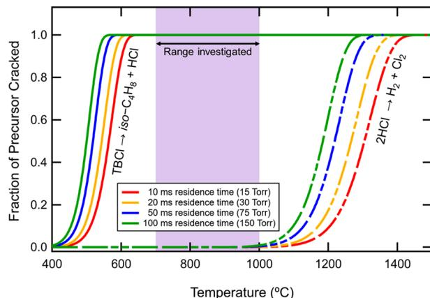
**FIG. 3.** Calculated fraction of TBCI and HCl pyrolyzed as a function of temperature based on typical residence times for precursors in the hot boundary layer above the substrate. The pyrolysis of TBCI into isobutene and hydrogen chloride (HCl) is fully complete by 600 °C, while the thermal decomposition of HCl does not occur until over 1000 °C.
