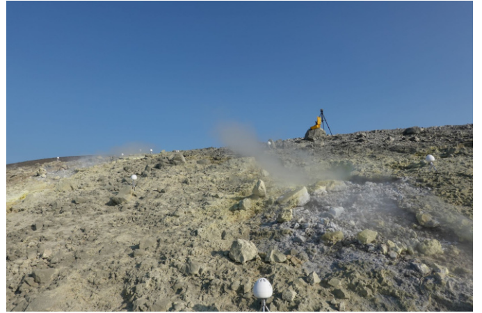
Fig. 1: Sensor eggs deployed on the fumarole field of the volcano “La Fossa”, Vulcano, Italy.
