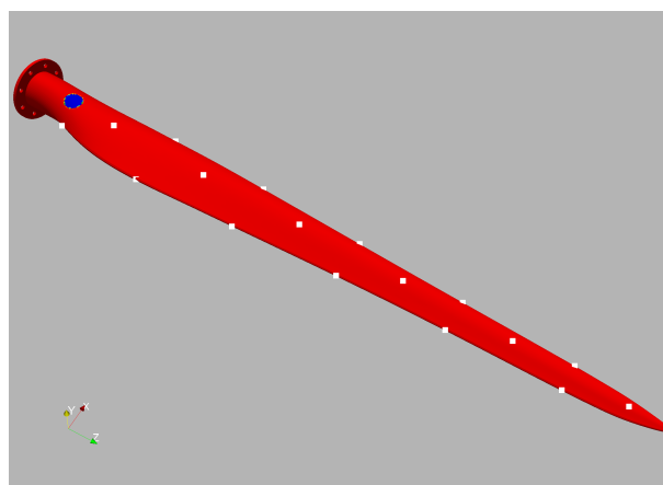
Figure 5.4d Weakened Region and Measurement Points
