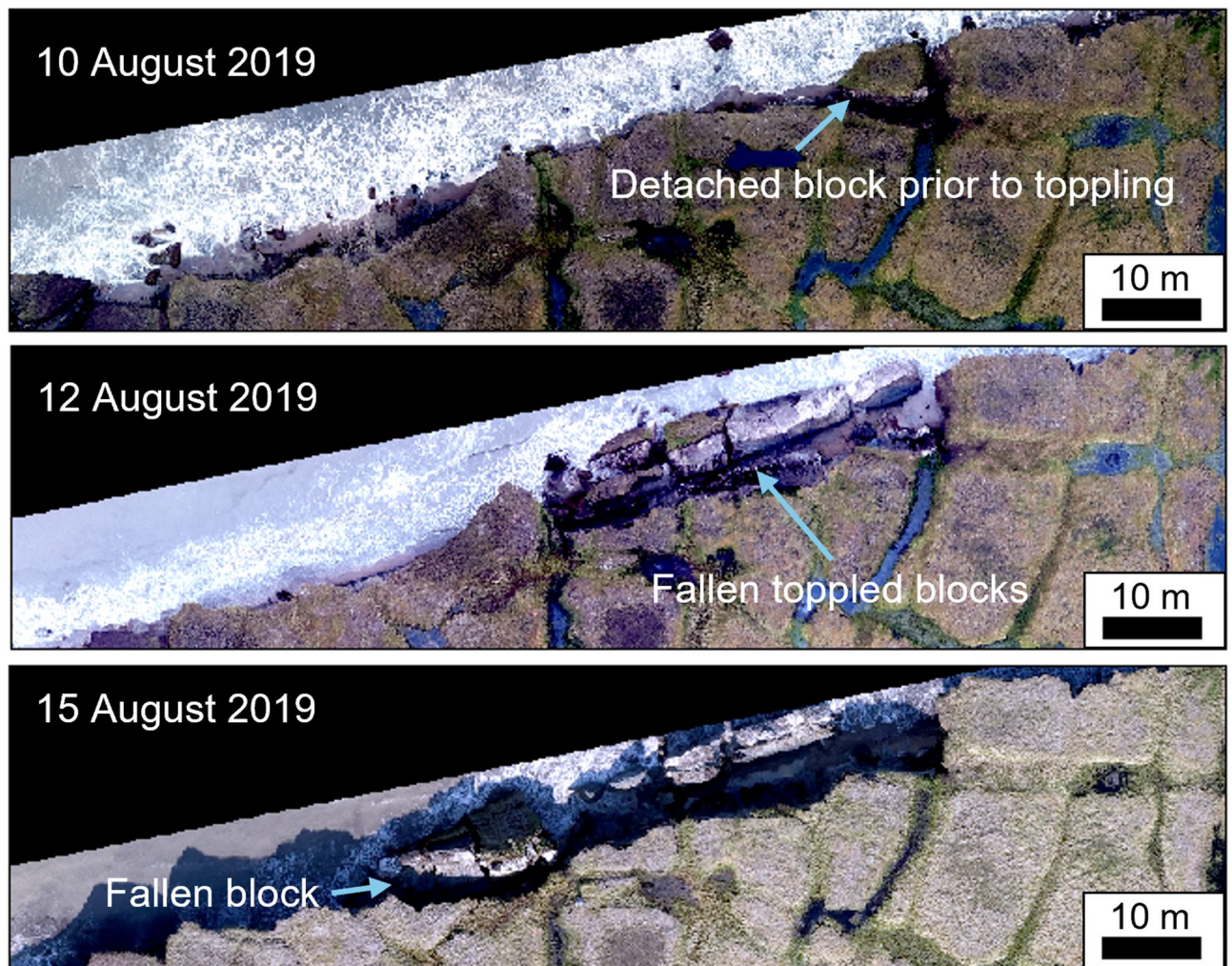
Fig. 4. Three consecutive timesteps of UAV imagery (10, 12 and 15 August) showing the same sub-section of coastline during the 2019 open water season. The timesteps show a section of coast where block failures occurred in three successive timesteps. The failures occurred from an east to west direction. These failures likely represent post storm lag of block failure from a storm that occurred within the 30 July to 2 August timestep.
