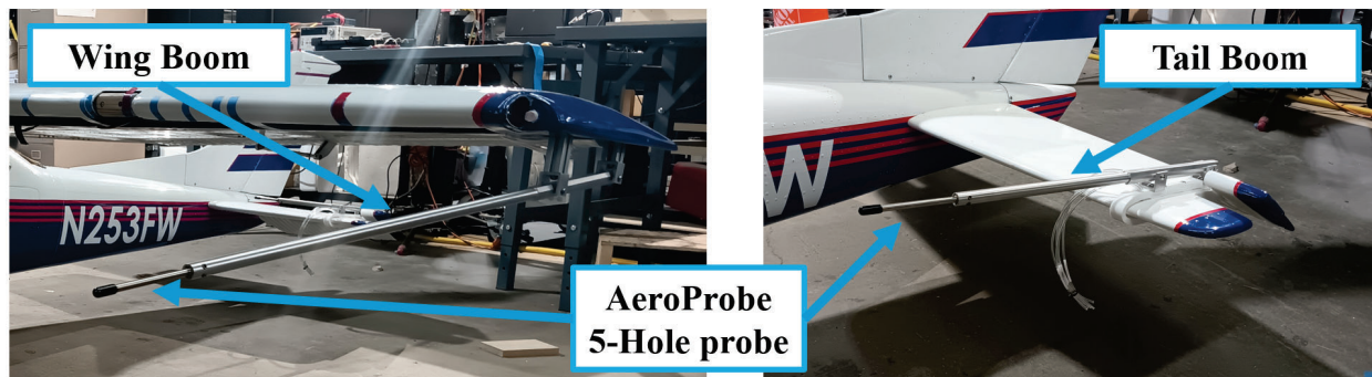
Figure 21. Air data booms and probes.
