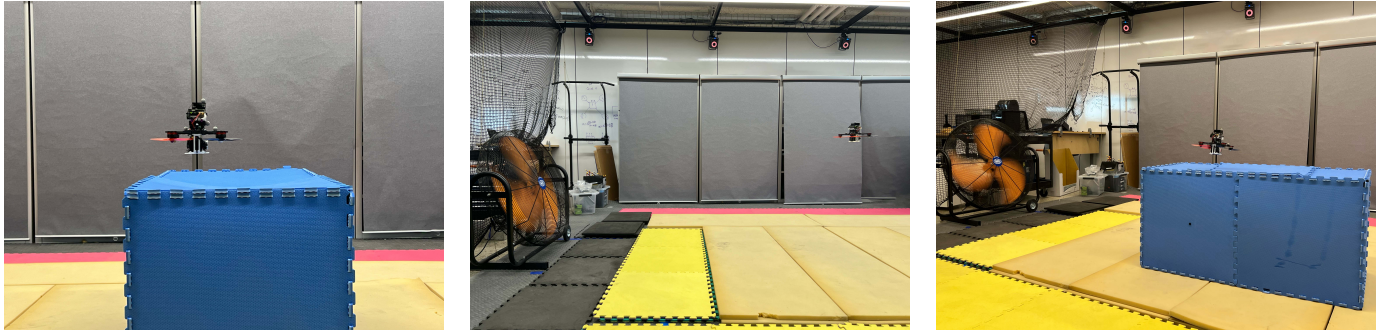
Fig. 1: Simultaneous System Identification and Model Predictive Control: Tested Scenarios of Reference Trajectory Tracking subject to Various Unmodeled Aerodynamic Disturbances. In this paper, we focus on simultaneous system identification and model predictive control where the robots' capacity to achieve accurate and efficient tracking control is challenged by unknown both dynamics and (possibly state-dependent) disturbances. For example, the ability of a quadrotor to track a reference trajectory can be challenged by a variety of unknown aerodynamic disturbances: ground effects (left & right), wind disturbances (center & right), and drag (all). We provide a control algorithm that demonstrates an ability to simultaneously learn such unknown dynamics/disturbances in a self-supervised manner, based on the data collected on-the-go, and uses the learned models for predictive control. We prove that the algorithm guarantees bounded suboptimality against the optimal controller in hindsight, under technical assumptions that we describe later in the paper.
