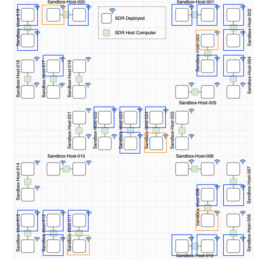
Fig. 5. ARA sandbox, with gNBs and UEs marked in orange and blue colors respectively
