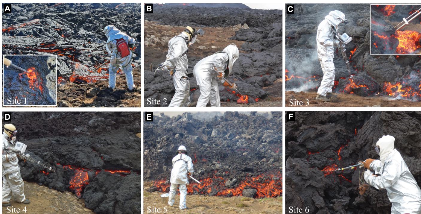
Figure 2. Field photos of six sites where viscosity and temperature measurements as well as sampling were performed. (A) Site 1, using rotational viscometer within sheet pāhoehoe lavas. (B) Site 2, sampling of spiny pāhoehoe lavas. (C) Site 3, using lava penetrometer within spiny pāhoehoe lavas. (D) Site 4, using lava penetrometer within transitional spiny pāhoehoe lavas. (E) Site 5, sampling lava on rubbly 'a'ā flow front. (F) Site 6, performing temperature measurement on 'a'ā lava flow front.
