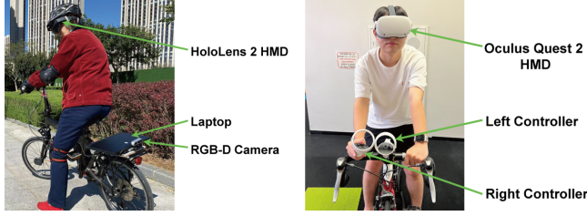
Figure 2: Images of the ReAR bicycle setup, including the HMD, RGB-D camera, and laptop from the rear view (left) and a participant with the bicycle and HMD used for the VR-based experiment (right). For the experimental apparatus, the left-hand controller was mounted to the middle of the handlebar for steering and the right-hand controller was mounted to the right side of the handlebar for input.
