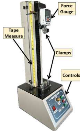
Figure 2. Force gauge and tower setup for tensile testing.
