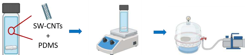
Fig. 3 Preparation Process of the Sensor: Development Stages.
