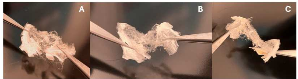
Figure 2. Images showing the fibrous textures of the SILS100-Electrofiber complex after the electro-spray procedure (1:10 silymarin: Eudragit® S100 ratio), showing the solid nature of the final product. (A) Complex after the electro-spray. (B) the complex is twisted using a pair of tweezers. (C) Stretching the complex.
