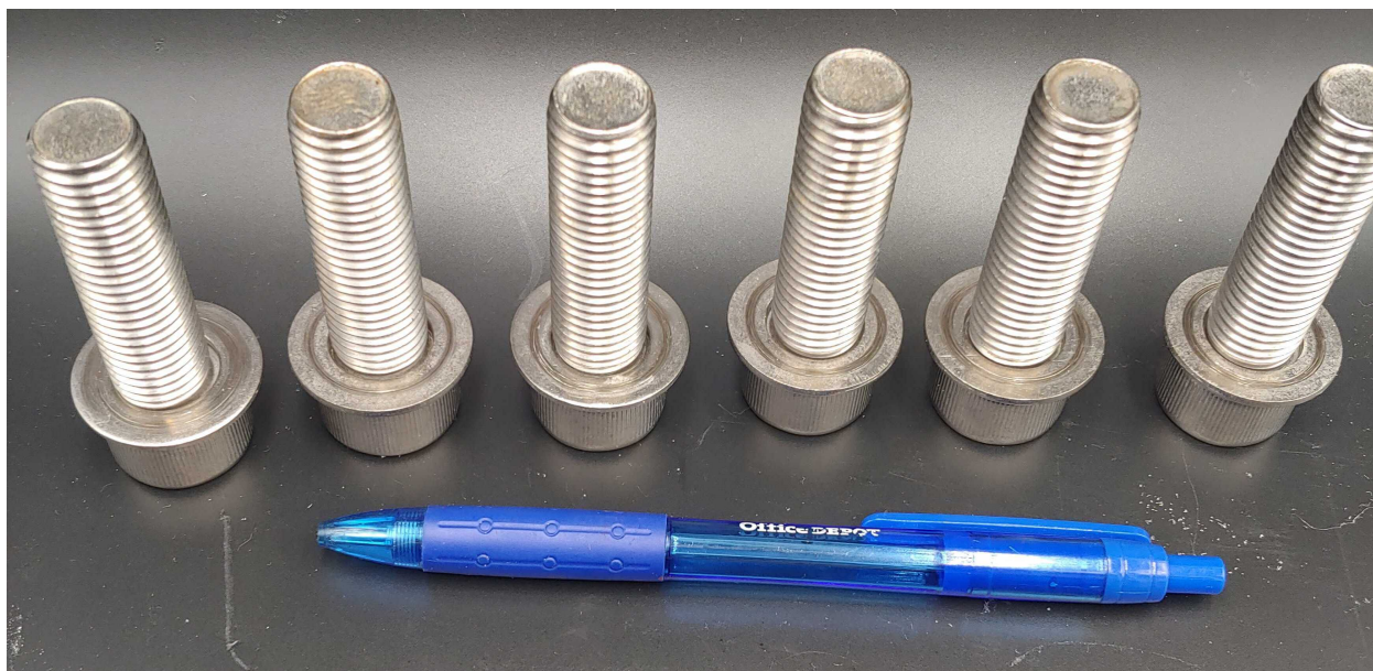
Figure S1 Bolts used to hold hold reactor head in place to the reactor body. For size reference, a pen is included.
