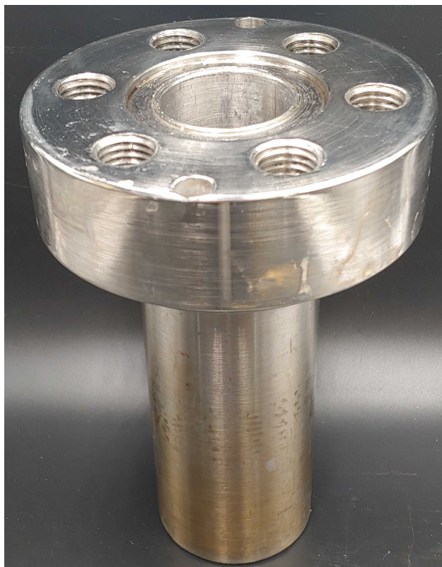
Figure S4 Photo of the 100 mL reactor body, with placement for 6 bolts. The inner ring is the metal gasket, crucial for a good, high temperature seal.
