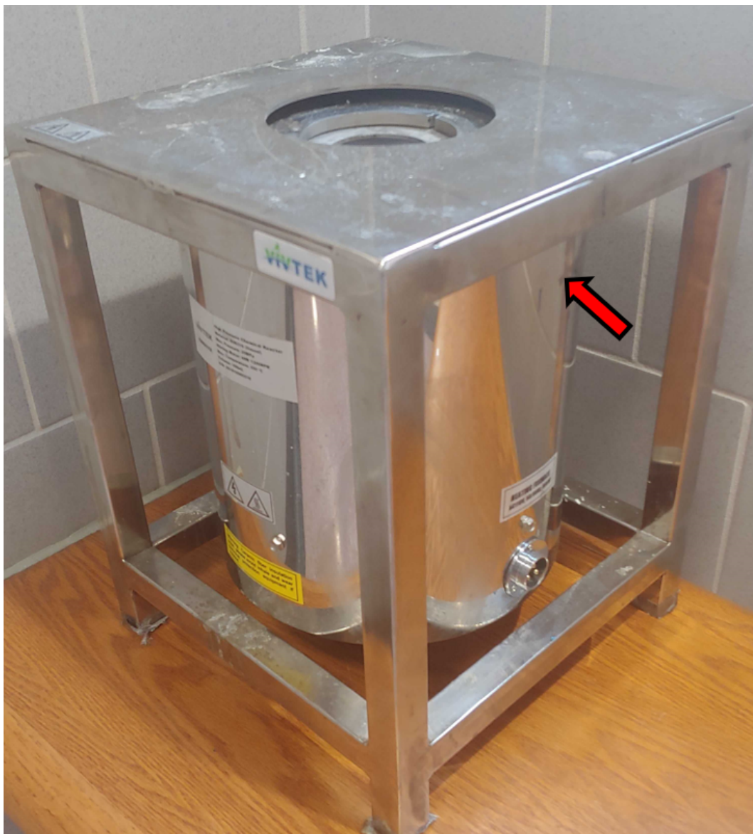
Figure S9 Photo of the furnace purchased from Vivtek. The arrow points to the location of the small hole drilled in the side threading between the heating coils. It is here the thermocouple is threaded into the chamber and placed on the outside of the reactor vessel.
