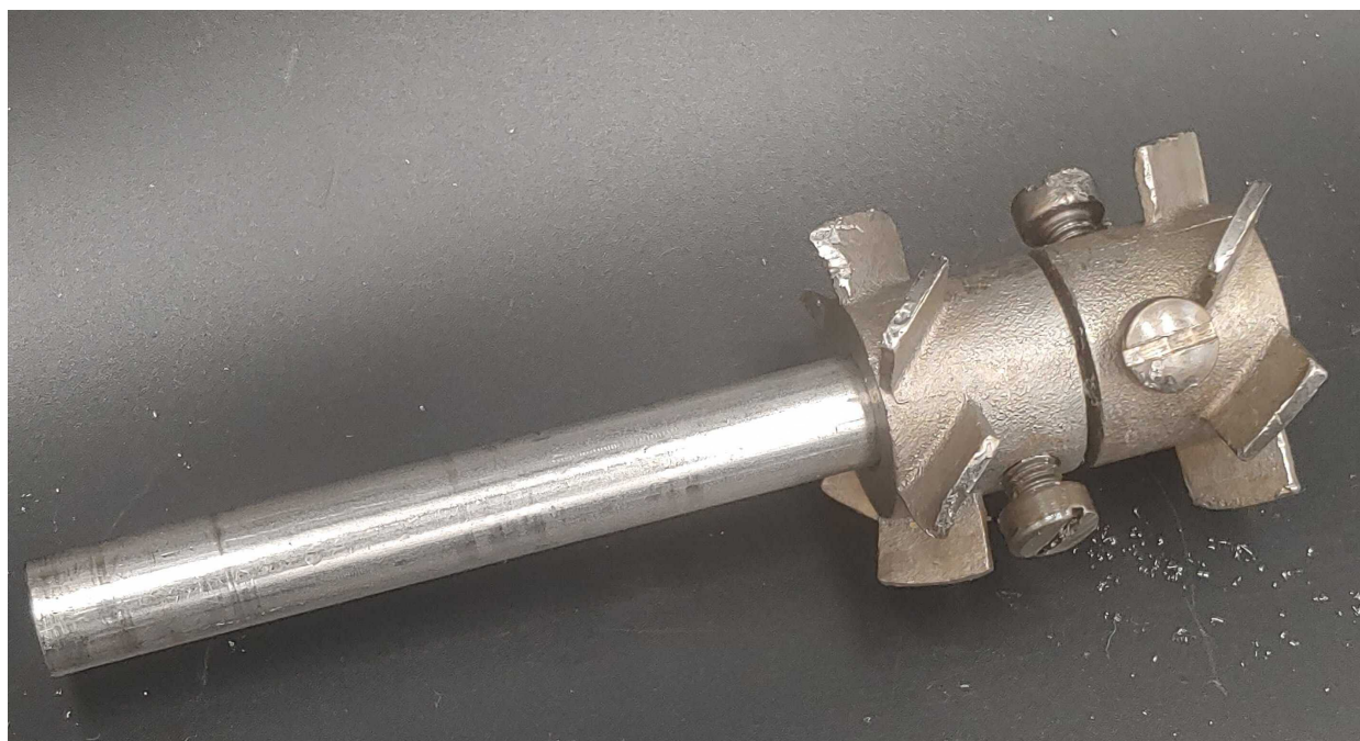
Figure S8 Photo of the agitator. The top is tapped, allowing the agitator to be screwed on and off. The blades are angled in opposite directions, allowing for thorough mixing.
