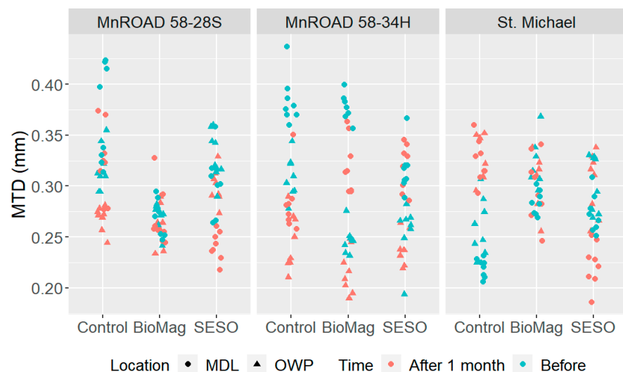
Figure 8. Macrotexture evaluation of the treated and untreated sections with Sand Patch test.
