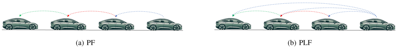
FIGURE 2. Typical IFTs for a platoon: (a) Predecessor Following (PF); (b) Predecessor Leader Following (PLF).
