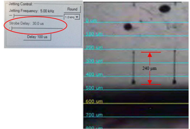
Fig. 5. Ink droplet travel for a strobe delay of 30 μs.
