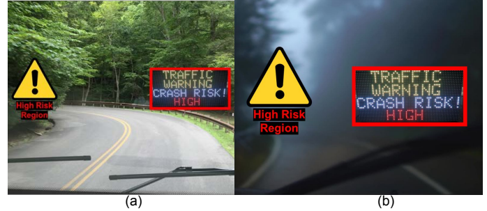
Fig. 1: IoT-based crash notification system is strategically implemented in hot-spot region, identified by thorough analysis of historical data. This system dynamically assesses and presents real-time crash risk, incorporating both static and dynamic information. High-alert notifications are triggered in instances where (a) unexpected obstacles significantly elevate the risk of traffic crashes and (b) adverse weather conditions or poor road conditions pose an increased threat to traffic safety.
