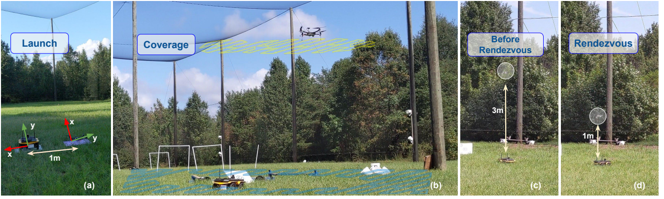
Fig. 5. Proof of concept field trials with VOXL m500 UAV and Clearpath Jackal UGV at Fearless Flight facility (F3) at University of Maryland, College Park, MD, USA. (a) The vehicles are launched from a predefined location with 1m offset between their origins. (b) UAV and UGV are performing coverage tasks until they reach the rendezvous location. (c) Before rendezvous each of the vehicles waits for the other one to arrive at the location, UAV is at the flight altitude 3m . (d) If both arrive UAV will rendezvous by descending to 1m altitude.
