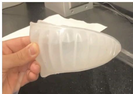
Figure 3: Silicone mold in the shape of the body of the fish.
