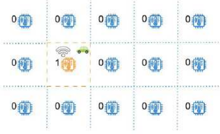
Figure 2: The graphic represents a strawman protocol in the boolean coverage model, where each sensor has a fixed sensing range and holds the coverage responsibility for a given area (marked by dotted lines here). The orange sensor detects the car in its sensed area and sends value 1 through gossip to the network, and every other sensor sends 0. Each sensor outputs the orange sensor's location as the target's location.
