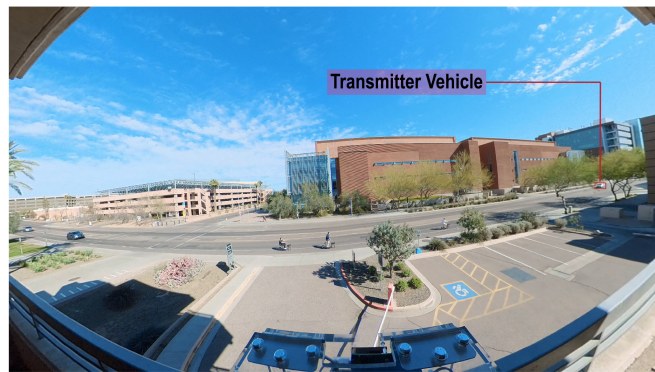
FIGURE 15. The mobile vehicle observed from the basestation at about 10 m from the distributed node of Unit 2. Within the 10-20 m range, some trees partially obstruct the LOS path between the basestation and the mobile vehicle, leading to a degradation in beam prediction for Unit 2 in this range.
