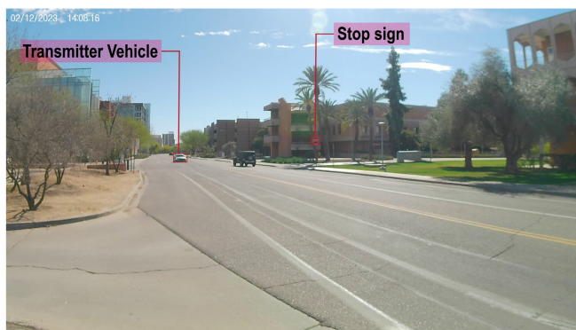
FIGURE 16. The mobile vehicle as observed from the distributed node of Unit 3. The vehicle is approximately 65 meters away from the distributed node. Upon reaching this distance, it stops at a stop sign and then accelerates. This acceleration makes it challenging for the machine learning model to predict the beam at the 5 th time stamp.
