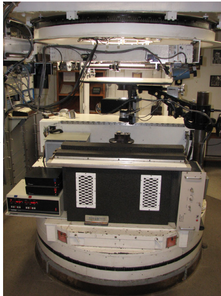
Figure 3 A photograph of the observation room taken by Larry Webster showing components along the optical path. This photograph was taken in 2007 after most improvements had been made. The guider ring at the top rotates to accommodate the optical axis set by the coelostat mirrors. The structure is driven by the X, Y screws which respond to the limb signal from the two pairs of sensors. The control of the image can be monitored by the out-of-focus image on the light baffle table. The filter wheel allows for the insertion of blocking filters or polarizer components. The K*DP polarizer is in a temperature-controlled box and provides variable isolation for the two circular polarization components. A table with drawing paper is inserted above the entrance aperture assembly to permit the daily sunspot drawing. The black box on the lid of the spectrograph holds the entrance aperture and the Walraven image slicer. Light enters the spectrograph through its slit after the image slicer.
