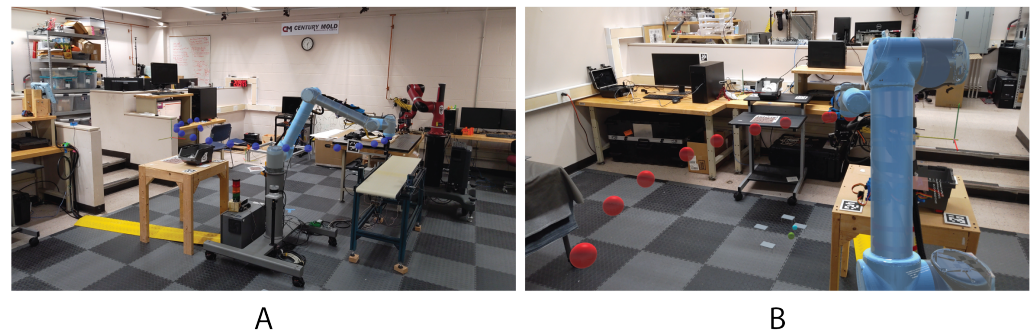
Figure 20. Spheres to show the robot end effector’s movement. (A) Blue spheres when the human is in a safe proximity to the robot. (B) Red spheres when the human is in close proximity to the robot.
