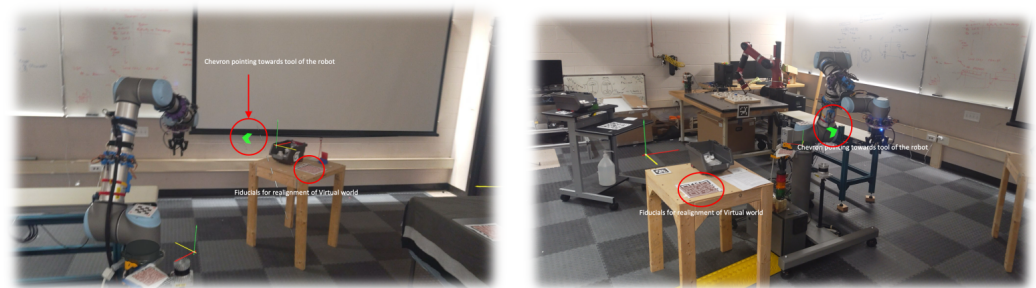
Figure 16. AR display shown to human workers through a HMD. Green arrow indicating robot's location is circled in red [123].
