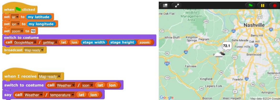
Figure 1. Simple NetsBlox project showing a map of our location as the background and displaying current weather conditions. Top script: stage, bottom script: sprite.
