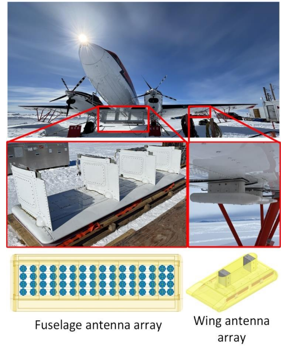
Fig. 2. Fuselage and wing antenna arrays photo/models.
