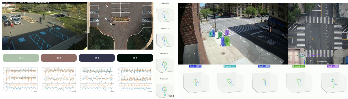
Figure 4: Visualization dashboard displaying live video, IMU streams, 3D bounding boxes, trajectories (camera and BEV views), and 2D/3D pedestrian poses, all processed via low-latency edge computing.
