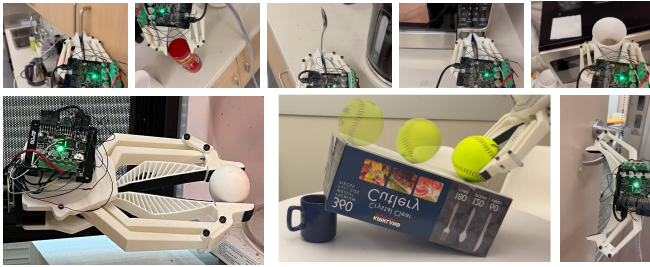
Fig. 6: Experimental evaluation for task versatility. BaRiFlex is mounted on a portable device and used by a human to perform multiple household tasks including a full long horizon activity, prepare a cup of instant coffee that involves tasks such as (top row, left-to-right): opening cabinets, opening jars, pinch-grasping utensils, pressing buttons, grasping delicate plastic cups. We also evaluated other tasks such as grasping an egg, catching a fast-moving object, and opening heavy doors (Bottom row). Through this human-controlled manipulation, we empirically evidence the high task-variability enabled by BaRiFlex, which covers a significant fraction of possible tasks in household domains.
