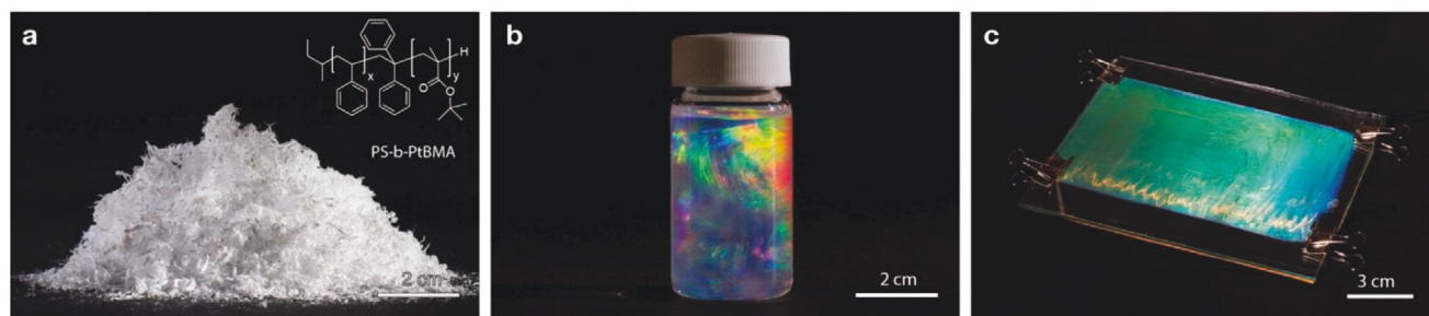
Figure 2. Different states of the block copolymer StB. a) Photograph of \approx 10 g dry StB after synthesis; Inset: Chemical structure of StB. b) StB in toluene solution in a 20 mL glass vial. Incident light from the right. c) A dry film of StB sandwiched between a glass substrate and a cover glass.
