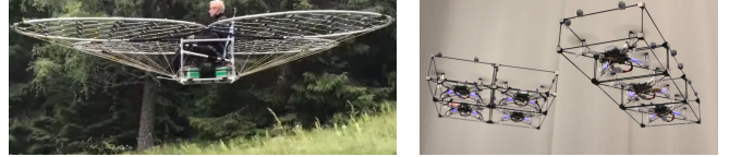
Fig. 1: (Left) The 76-rotor chAIR can lift a human [1]. (Right) ModQuad structures with 12 and 28 rotors [18]. All vehicles have redundant rotors.
