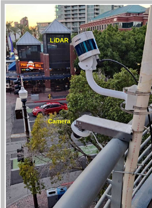
FIGURE 1 Data collection setup at downtown Tempe intersection.
